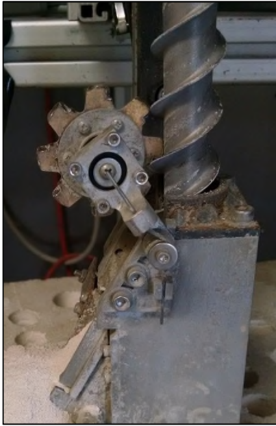
Figure 11. Keyed scraper for IceBreaker (a TRIDENT predecessor drill) [5].
