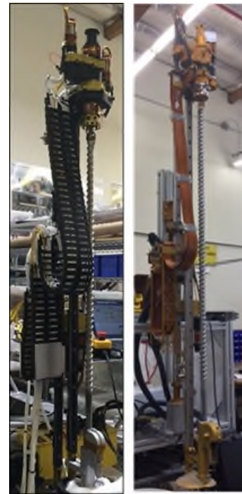
Figure 17. Reduced bulkiness and mass from RP15 (left) to TRIDENT (right).
