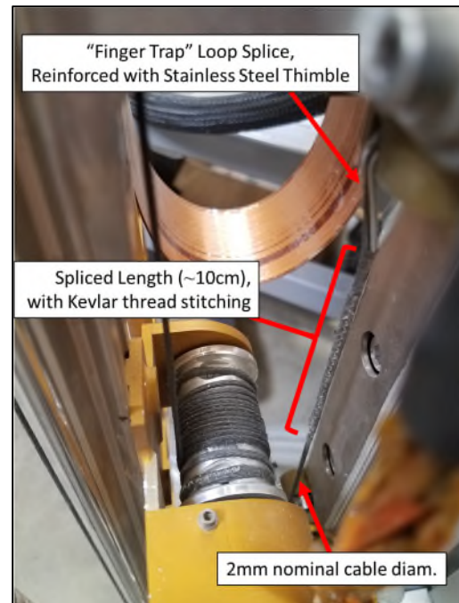
Figure 1. Technora cable termination and spool.
