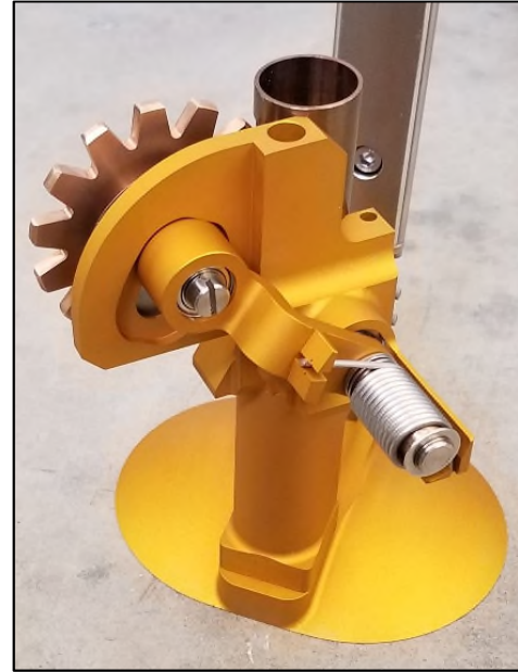
Figure 14. Alternative Support to use for brush (scraper shown here).
