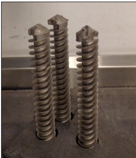
Figure 15. Assembled drill bits with deposited brazing paste in graphite support.
